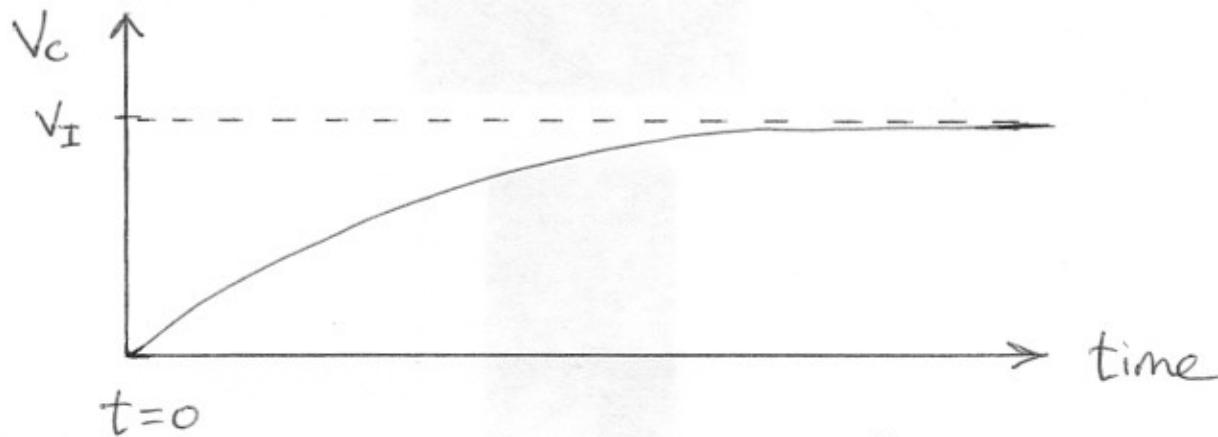
This is analogous to what is called a "step response" because the input to the system has a step input.
